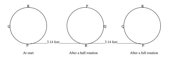
The car has moved forward  $\frac{\pi(1)(180)}{180} = \pi \simeq 3.14$  feet after the first half rotation. It moves another 3.14 feet after the second half rotation. Therefore it moves a total of  $2\pi \simeq 6.28$  feet when the tire makes a full
